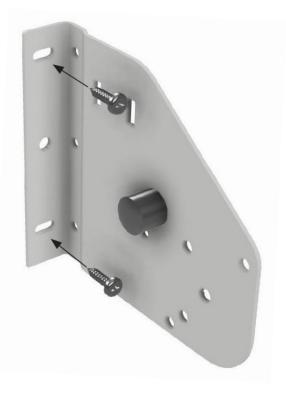
Attach mounting brackets with the appropriate screws (provided).
