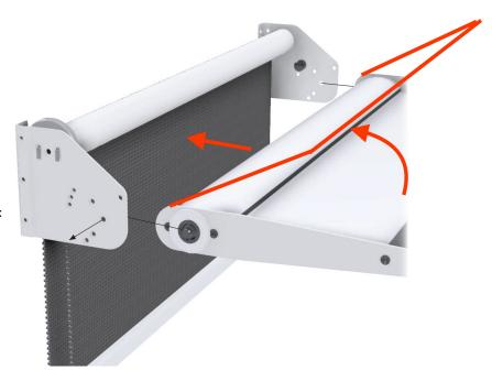
With the lightshelf held at an angle compress the spring-loaded pin-ends and slide it back into the "hockey stick" slots until it snaps in – slide the lightshelf back until the pin-ends seat into the end of the slot.
